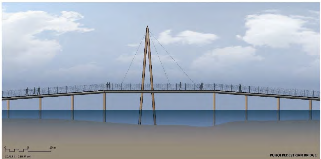
Initial rendering of the proposed Judge Arnold Turner Footbridge by Littoralis Landscape Architecture, focussing on the swing-opening span—‘this method is seen as having particular relevance as it reflects the mode of the historic bridge that once existed further upstream.’ (See also design outline and underlying principles, pages 16–17.)
